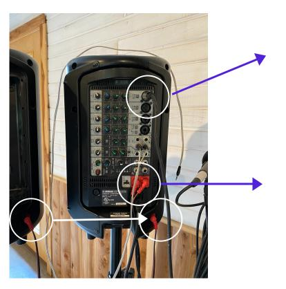
Mic input (make sure cord is also plugged into the microphone)
